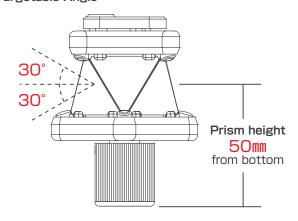
When using the prism pole (5/8-inch thread), please use the Prism Pole Adapter MAG2 (option).
